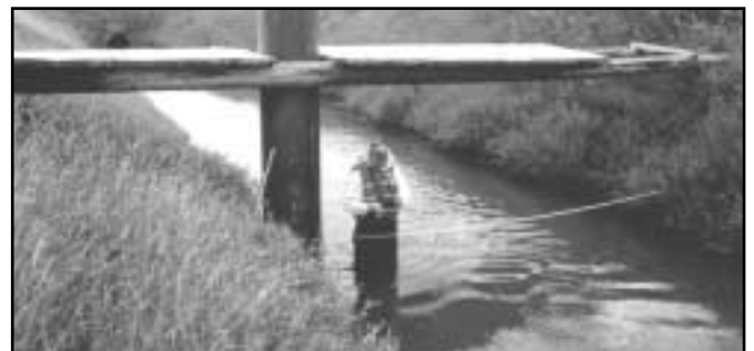
Figure 1. Flow measurement in the Battersea Drain.
